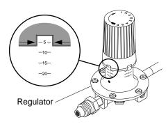
Figure 5 - Adjustable Regulator Set At 7 psig
